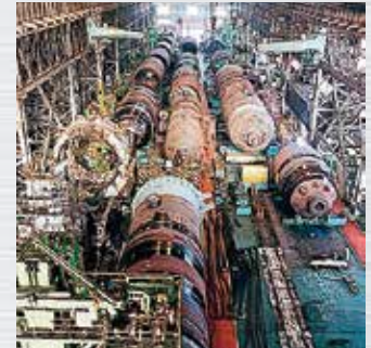
Pressure Vessel Welding Fabrication Line
