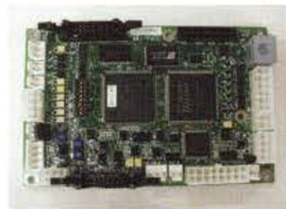
JSW original high-speed servo control board
